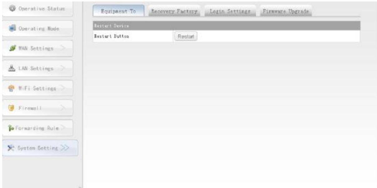
Restart equipment will set in after the change to take effect. After the restart, the device will automatically cut off the WAN port connection.
