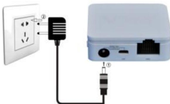
Picture 4-1 VAR11N Hardware installation diagram
