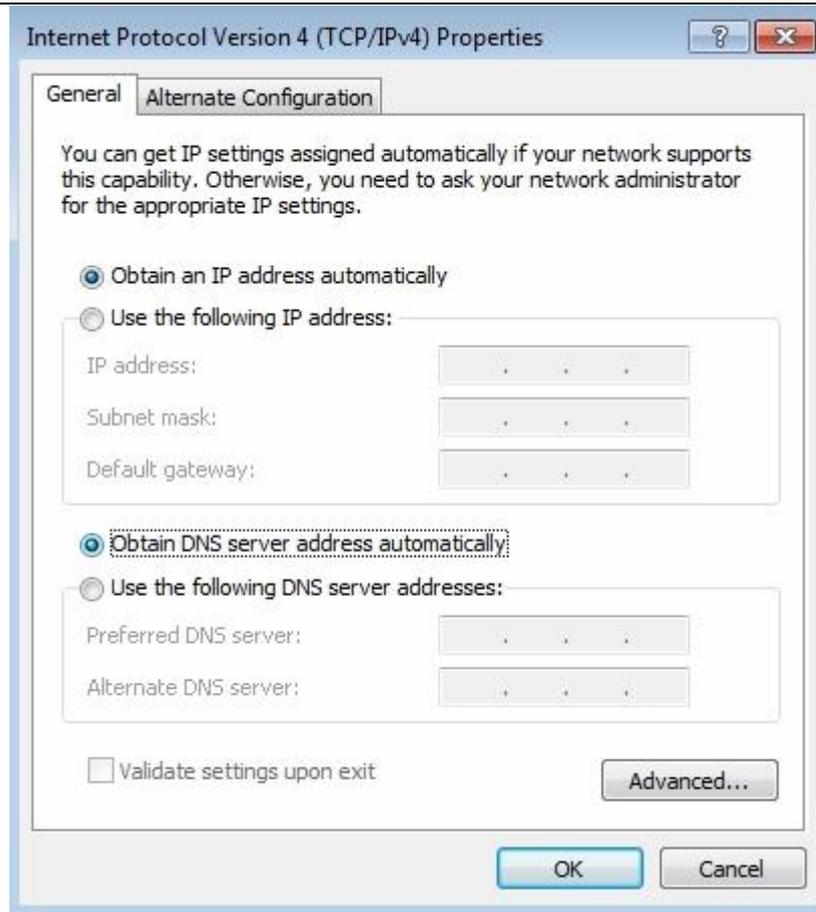
4. In WIFI Bridge mode, because VAR11N DHCP server is closed and can't assign IP address for computer, then you should configure the IP address for Local Area connection manually to login the webpage of VAR11N. The IP address of computer should be configured to 192.168.1.X ( $2 \leq X \leq 253$ ), the subnet mask to 255.255.255.0. Please see the following picture, click confirm. Return to the last interface, click confirm, please see the following picture:
