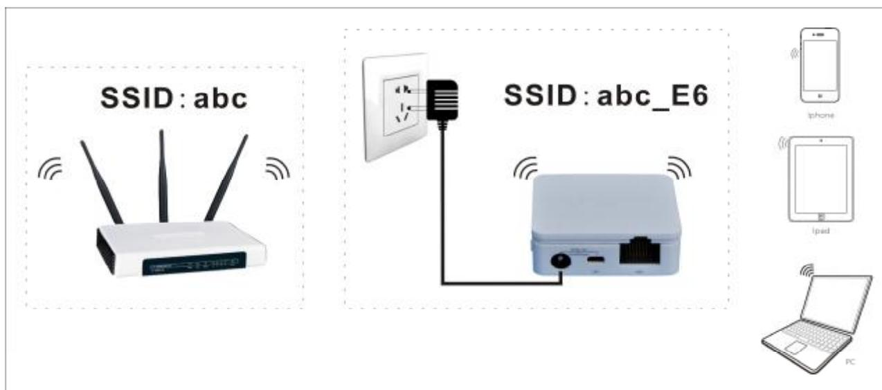
Picture 3-4 Bridge with AP Mode Connection diagram
